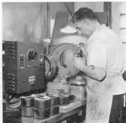
Figure 2. Typical installations of the \frac{3}{4} -hp Variac Speed Control, (left) on a lathe, and (right) on a toroidal winder.
